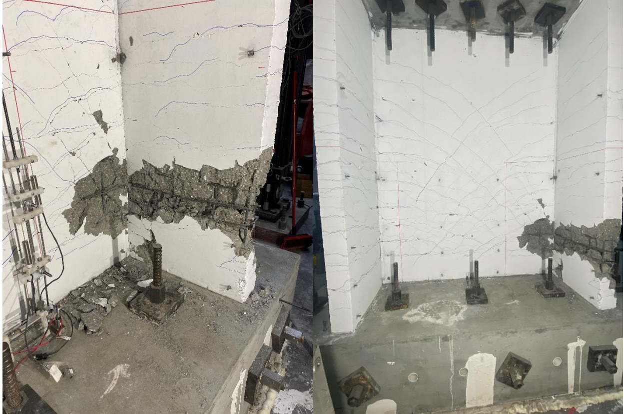
Figure 4-7: Inside surface of West flange (left) and the web (right), after the test
