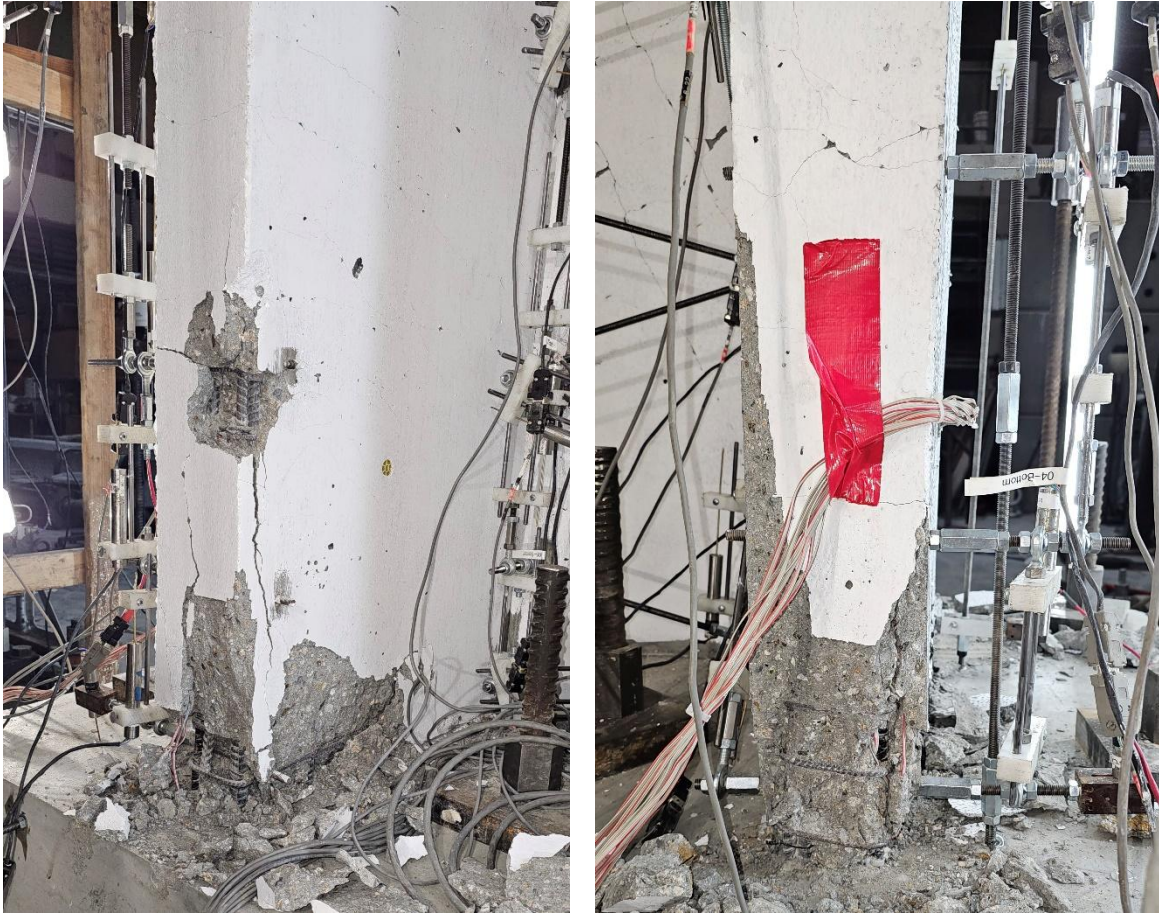
Figure 5-5: East flange edge (left), West flange edge (right) after inelastic ramp-down cycles of WLP, CW-2
