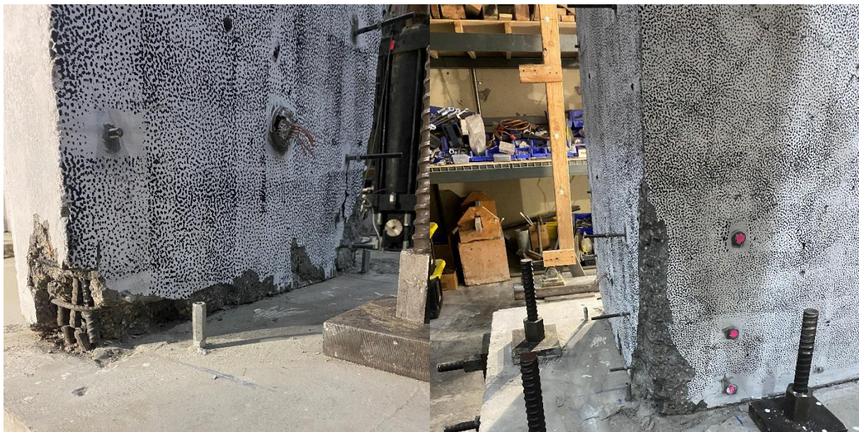
Figure 6-11: West flange edge (left) and west flange corner (right) after the completion of testing, CW-4
