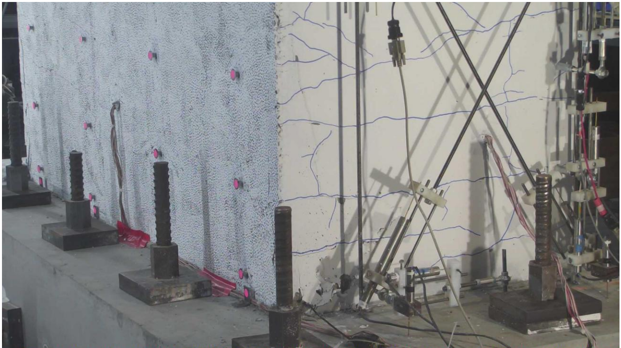
Figure 4-2: Damage state of the East flange and the web after two cycles at 1.5% hinge rotation demands (at zero loads)
