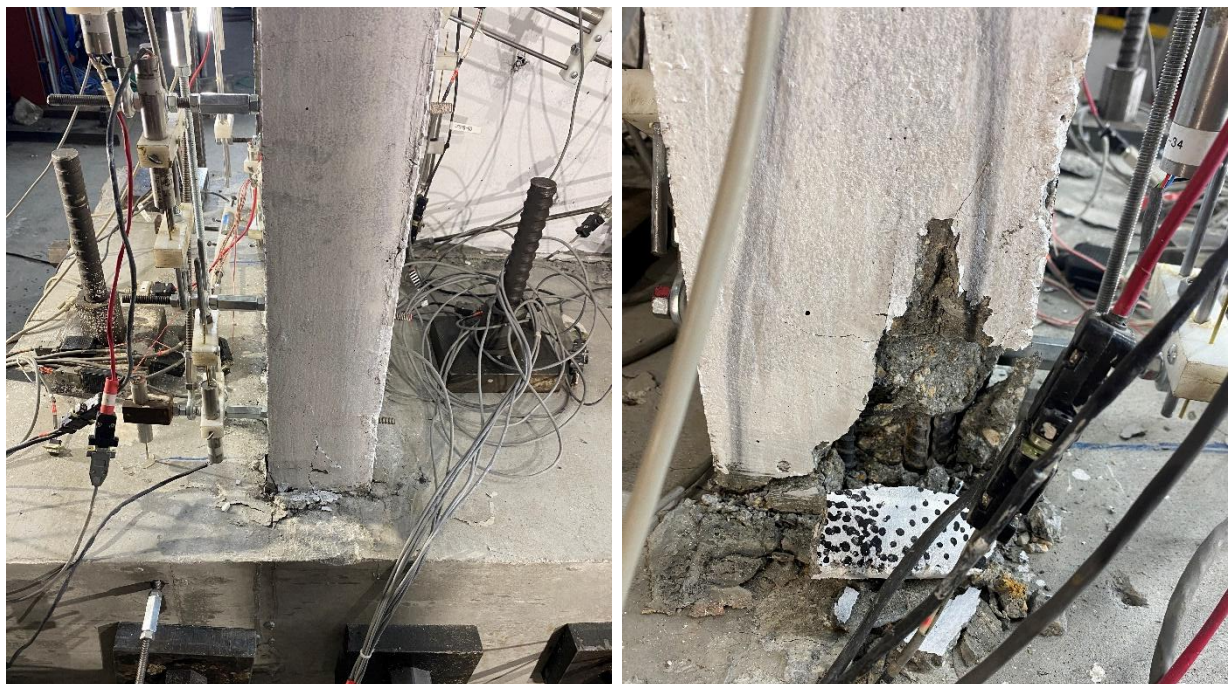
Figure 5-13: East flange edge (left) and West flange edge (right) after the ramp-up loading of WLP, CW-4
