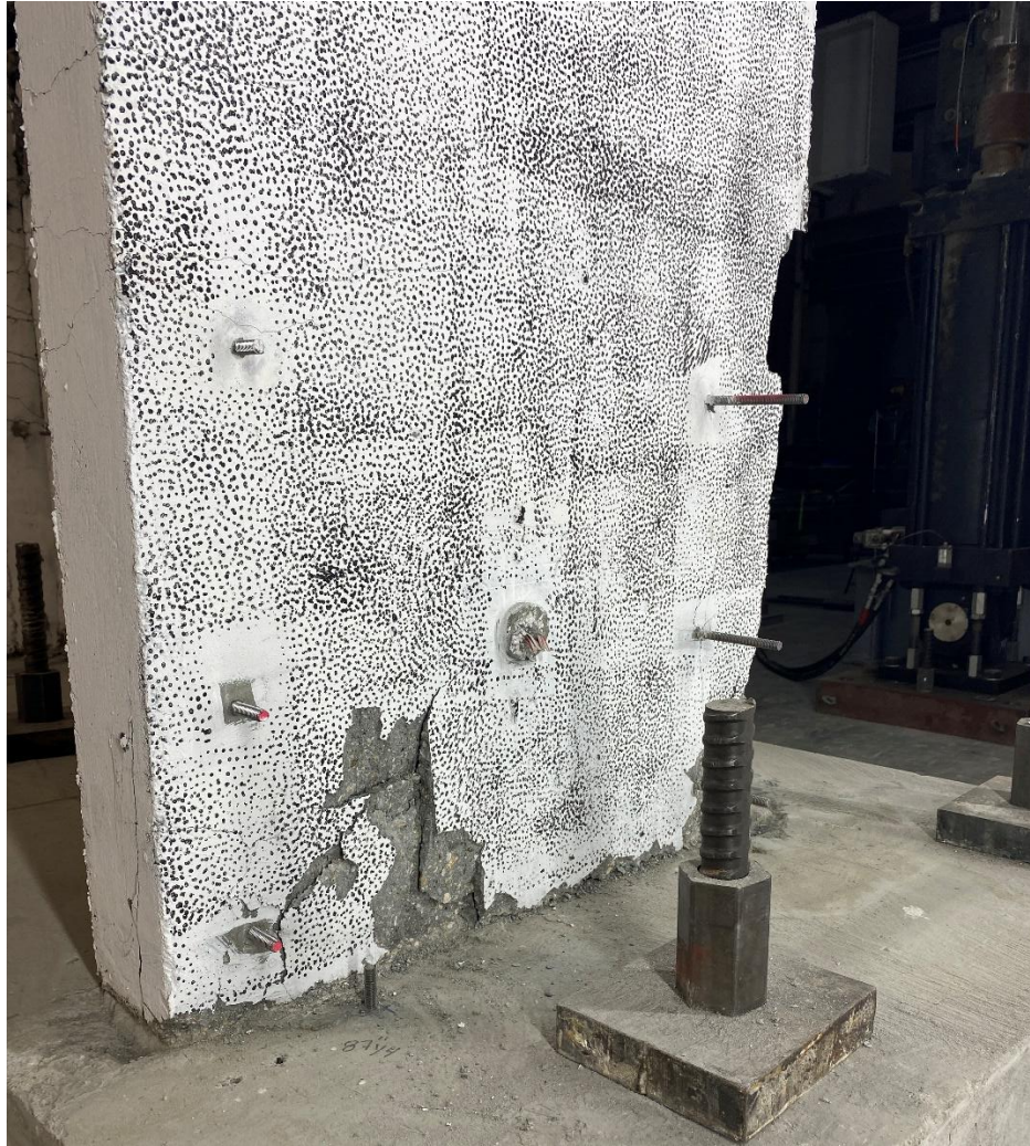
Figure 6-9: Damage state of the west flange after the completion of testing, CW-3
