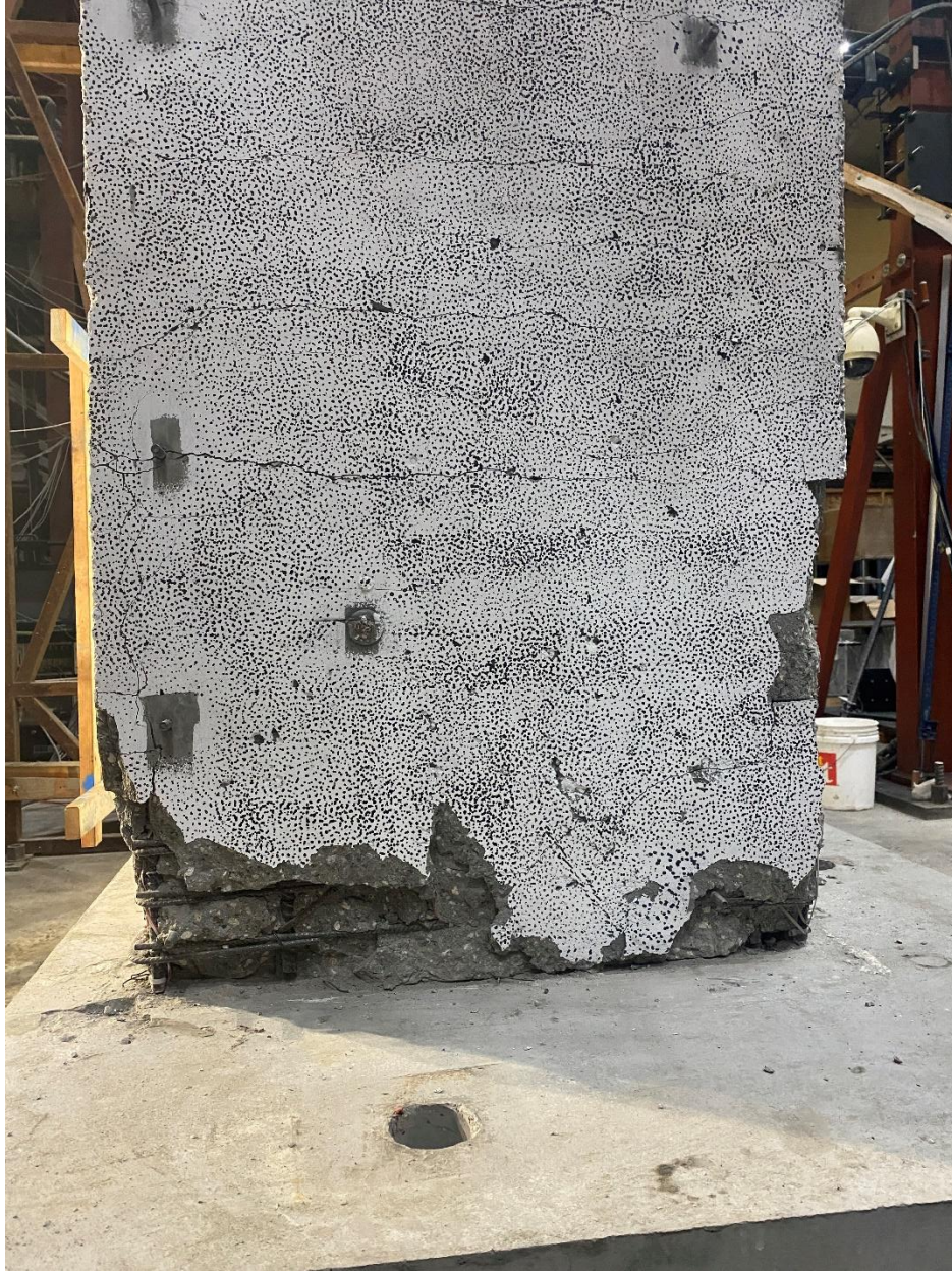
Figure 6-4: Damage state of the west flange after the completion of testing, CW-2
