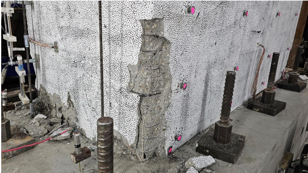
Figure 5-7: West flange after inelastic ramp-down cycles of WLP, CW-2
