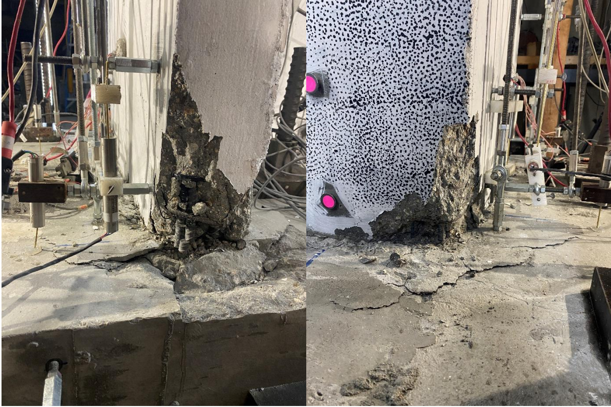
Figure 6-10: East flange edge (left) and east flange corner (right) after the two cycles applied at \pm 0.9\% IP hinge rotation demands, CW-4
