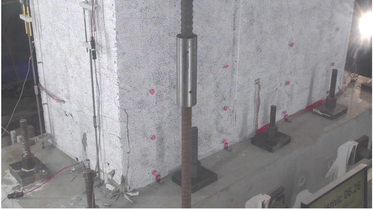
Figure 4-1: Damage state of the West flange and the web after two cycles at 1.5% hinge rotation demands (at zero loads)
