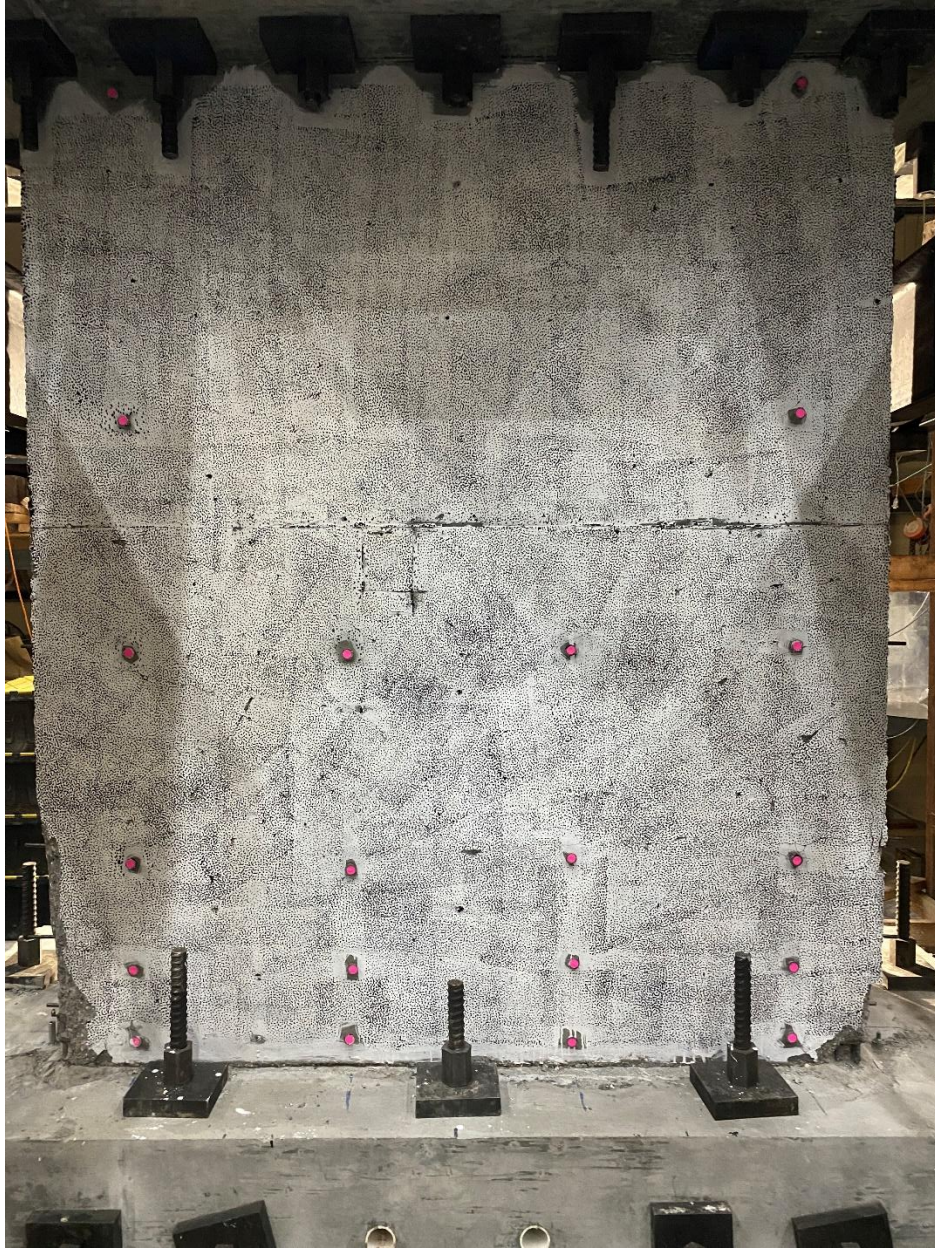
Figure 6-13: Outer surface of the web after the completion of testing, CW-4
