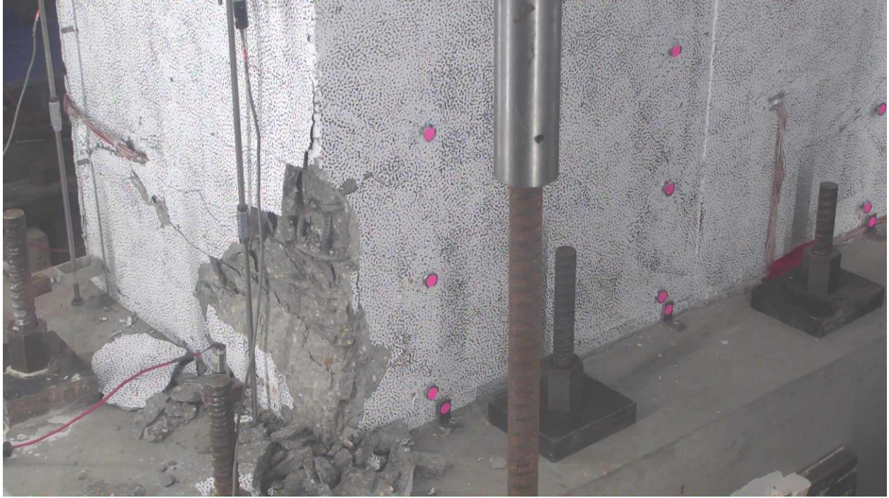
Figure 4-3: Damage state of the West flange and the web after the first cycle at 2.0% hinge rotation demands (at zero loads)
