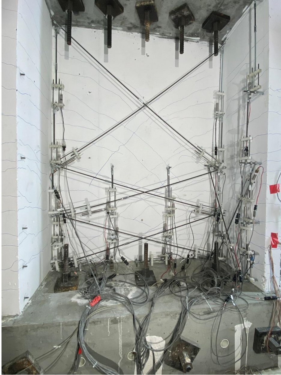
Figure 3-6: Cracking condition of CW-1 at the end of WLP (Inside surfaces of the web and flanges)
