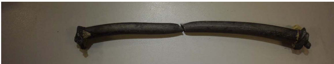
Figure 3-47. Tie bar fracture during testing of Specimen C2
