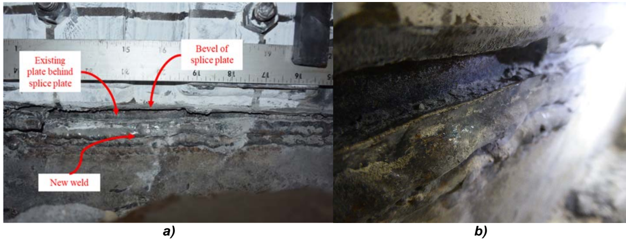
Figure 4-23. Close-up pictures of the fracture propagation at SWS from: a) front view and b) side view
