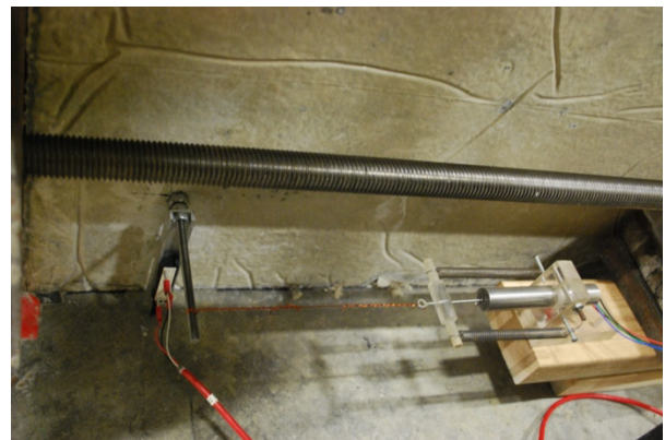
(f) Displacement transducers to monitor potential wall uplift and slip
