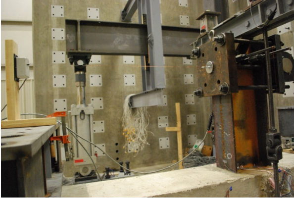
(a) External displacement transducer to measure beam deflection
