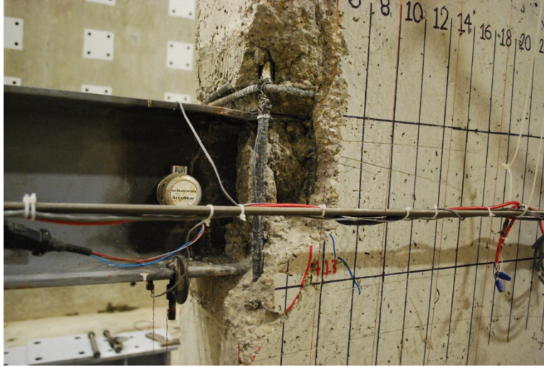
Figure 3.8 Condition of connection at the conclusion of wind load protocol tests – specimen 2a (test 3).
