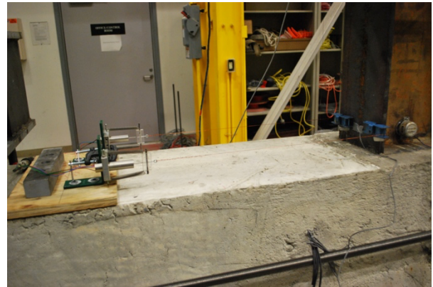
(d) Displacement transducers to measure deflection of the beam near its base
