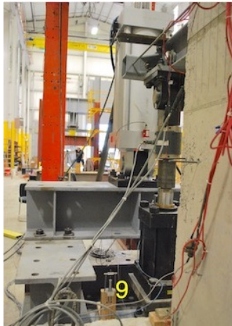
(c) 9: additional measurement of beam deflection at load point
