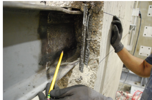
(b) Flange bending and web buckling
