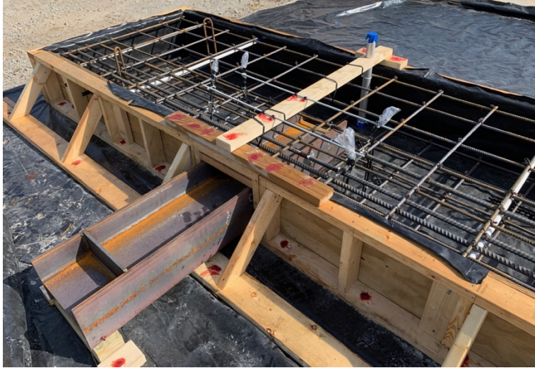
(a) Specimen 4 (test 6) [specimen 3 (test 5) was similar but with a shorter embedment length]
