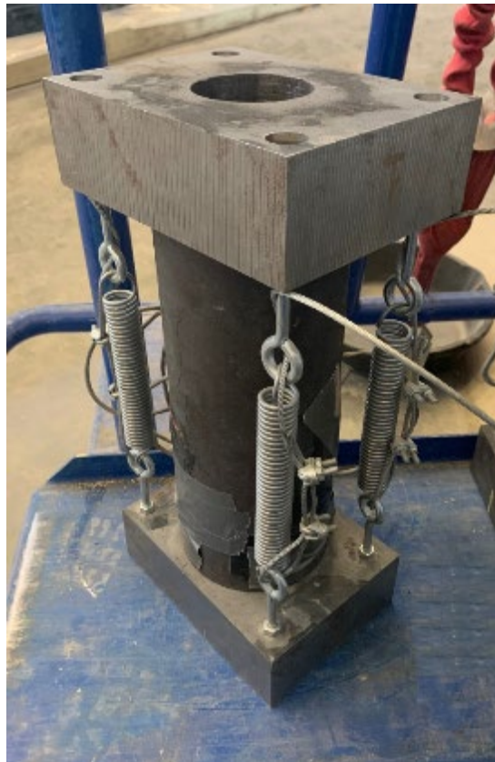
Figure 2.23 Load cell for No. 14 and No. 18 bars
