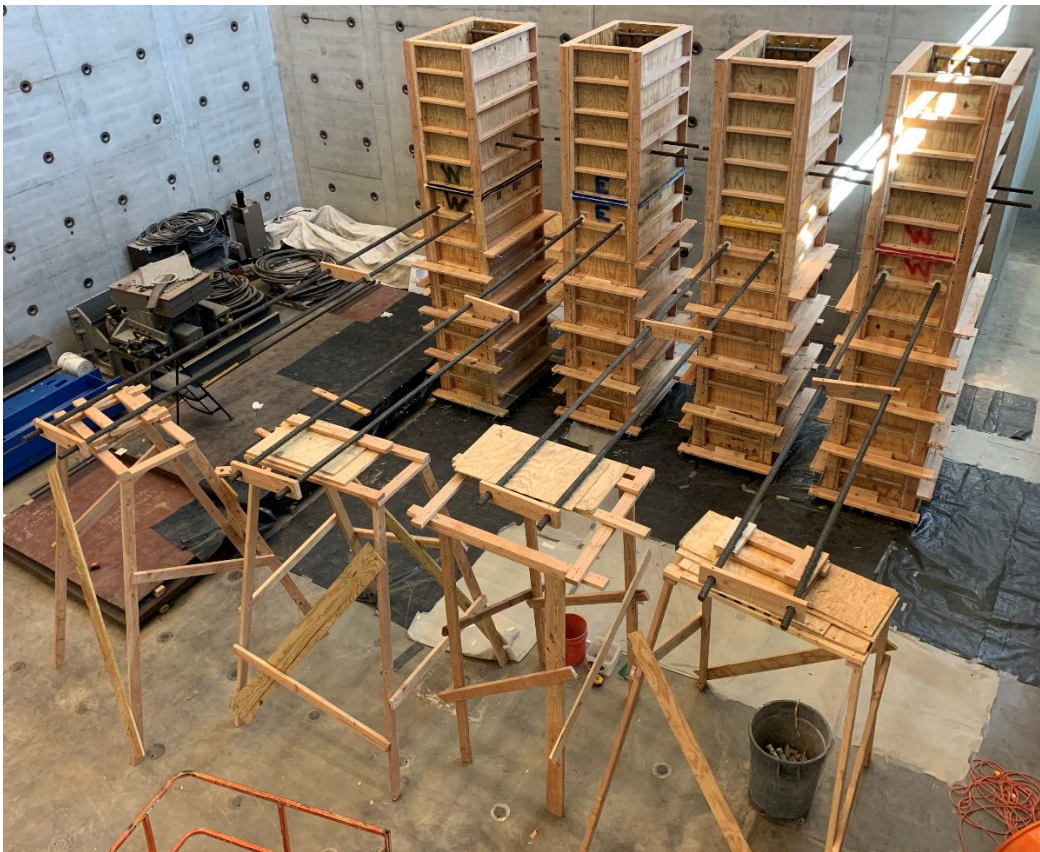
Figure 2.8 Vertical formwork for No. 14 bar specimens and sawhorses to hold the bars
