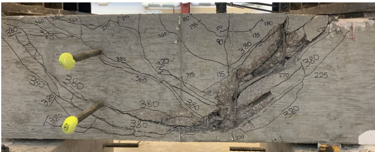
Figure 3.10 Concrete breakout accompanied by side splitting and compression failure of concrete between bearing face of the head and lower bearing member (specimen 14-16B)
