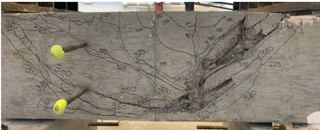
Figure 5.20 Anchorage failure observed in specimen 14-16B ( A_{tt}/A_{hs} = 0.178 ) tested under loading condition B
