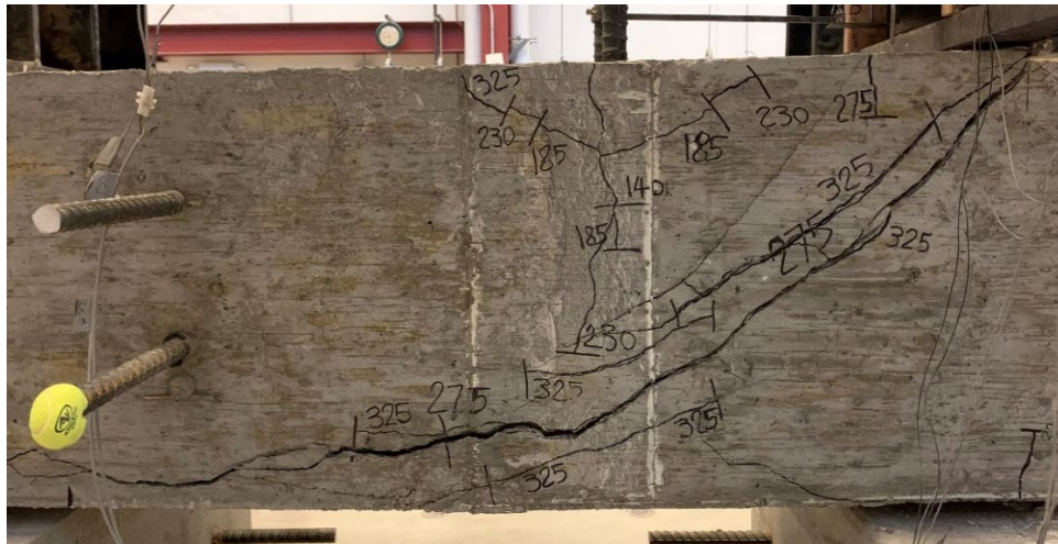
Figure 5.17 Shear-like failure observed in specimen 14-16A ( A_{tt}/A_{hs} = 0.178 ) tested under loading condition A
