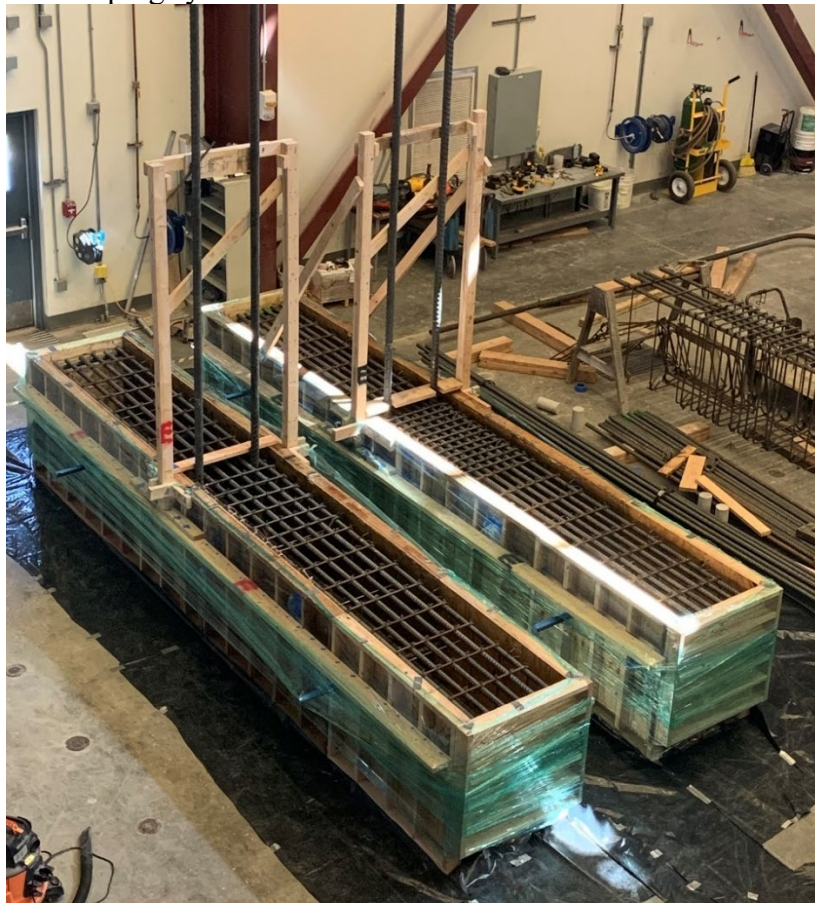
Figure 2.10 Horizontal formwork for No. 18 bar specimens
