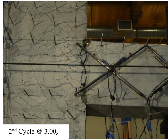
Figure 4.2. Damage Photos for SRC-W2 (continued)
