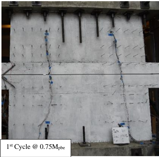
Figure 4.5. Wall Damage Photos for SRC-W1
