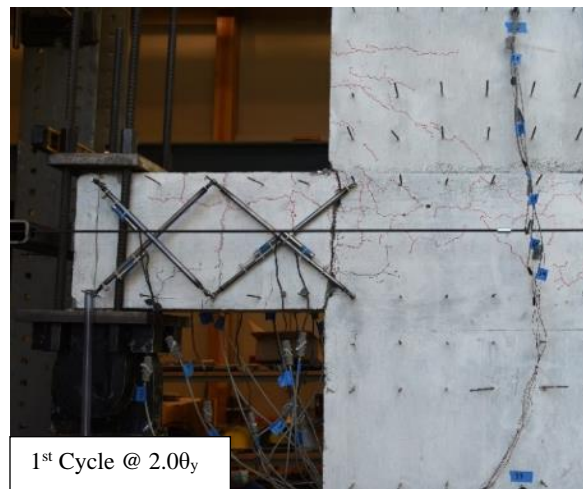
Figure 4.1. Damage Photos for SRC-W1 (continued)
