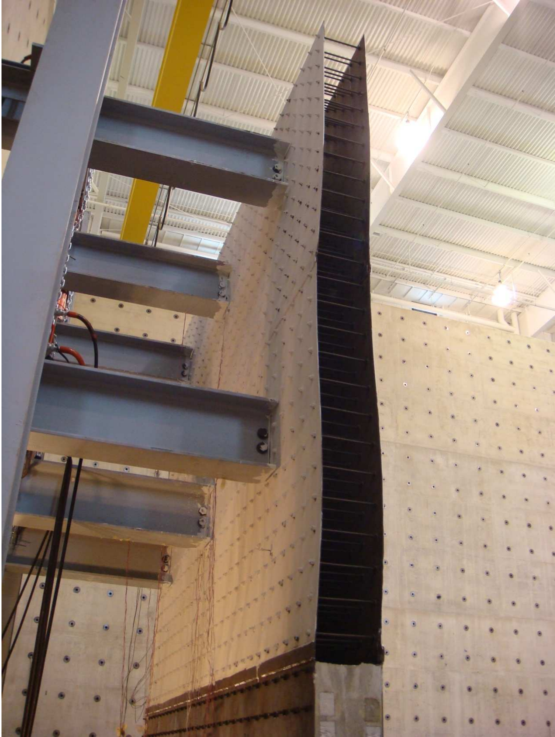
Figure 3.33 Distorted stability specimen at maximum applied load (168 kips) – View 2
