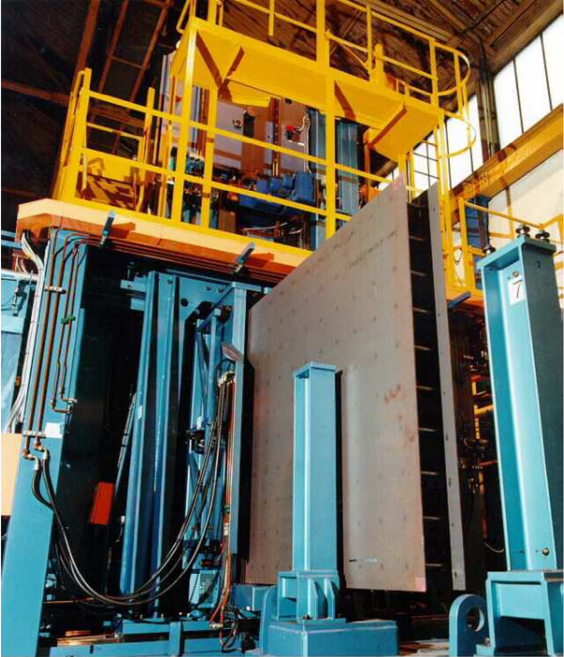
Figure 1.3 Fabrication of Bi-Steel panel assembly (Xie and Chapman, 2006)
