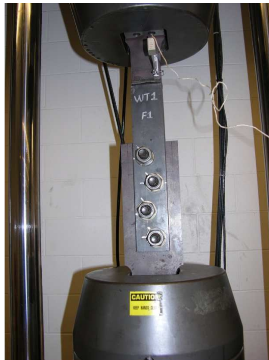
Figure C.6 Weld Joint Specimen Tests - Cyclic Loading in Four Pole MTS Testing Machine (Specimen 1)
