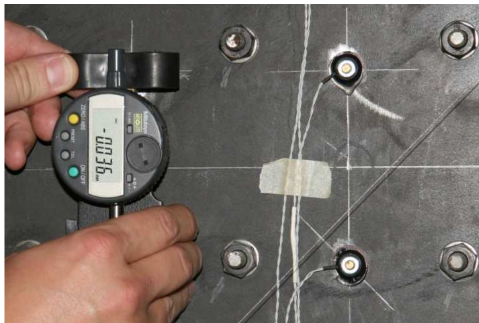
Figure 6.48 Invar beam with digital gauge over a pair of DEMEC points
