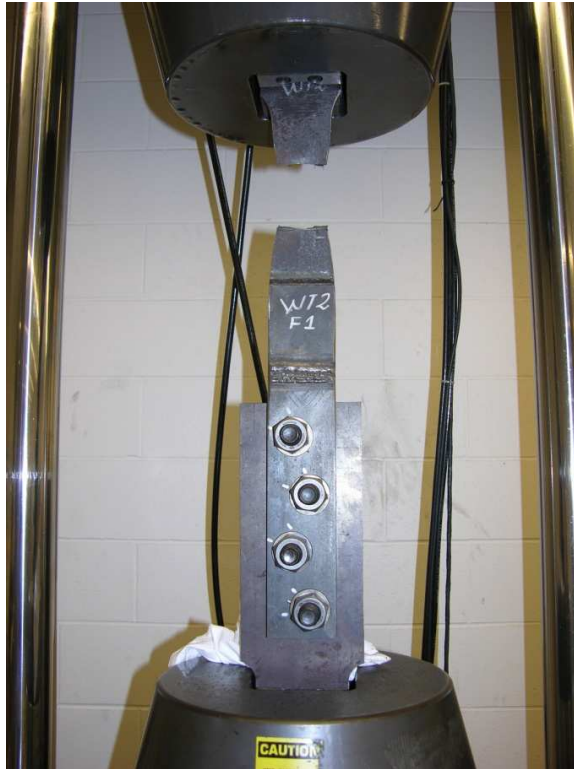
Figure C.9 Failure of the Weld Joint Specimen (Specimen 2)
