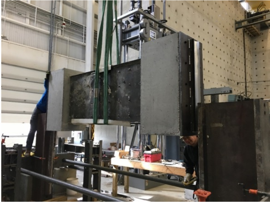
Fig. 2-5. Placing CW1 in the test setup
