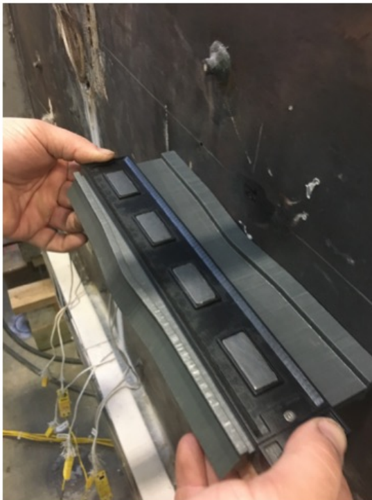
Fig. 2-15. Local buckling in CW1 specimen after the fire test
