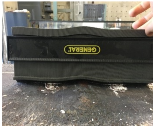
(d) Local buckling between shear studs at the top flange
