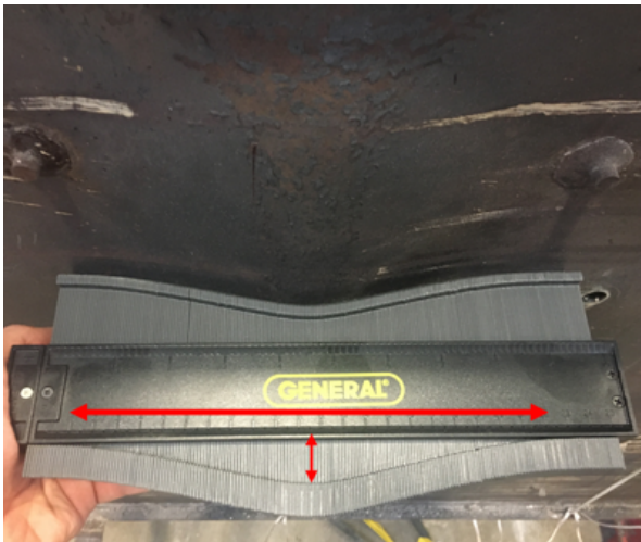
(c) Size of local buckling in CW3 with steel plate slenderness of 48
