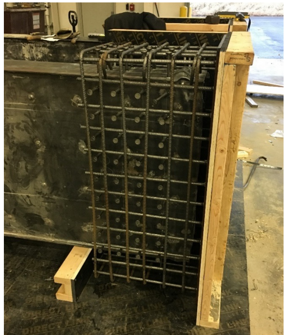
Fig. 2-2. (a) Specimen with welded headed shear studs (b) Concrete blocks steelwork
