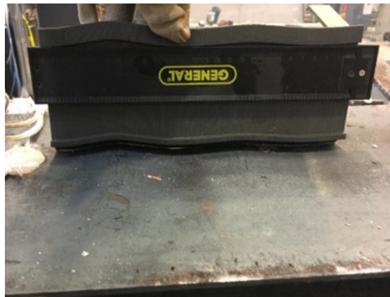
(d) Local buckling between shear studs at the top flange
