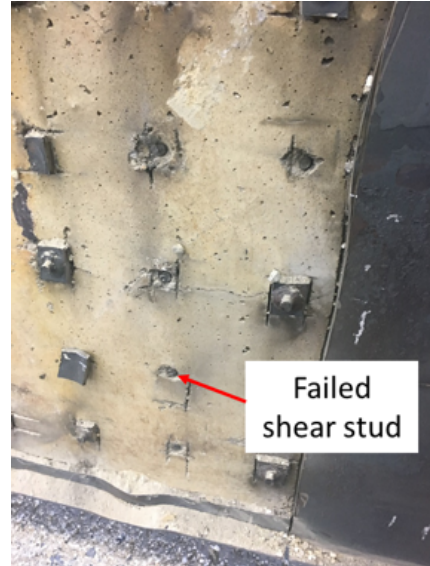
Fig. 2-19. Failed shear studs after the fire test
