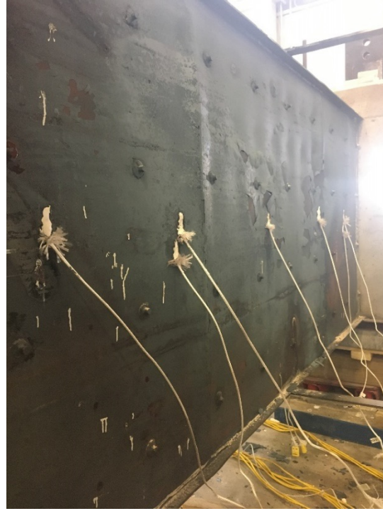
Fig. 2-15. Local buckling in CW1 specimen after the fire test
