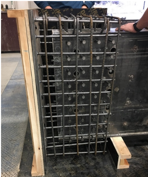
Fig. 2-2. (a) Specimen with welded headed shear studs (b) Concrete blocks steelwork
