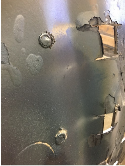
Fig. 2-19. Failed shear studs after the fire test
