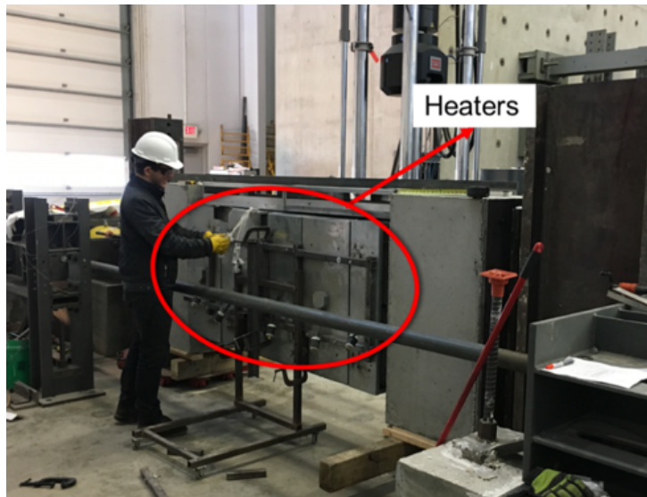
Fig. 2-8. CW1 located in the test setup ready to test
