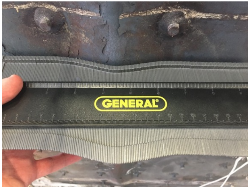
(b) Local buckling in the specimen
