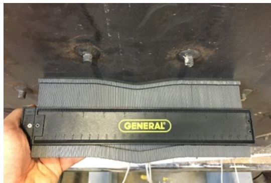
(c) Local buckling between tie bars
