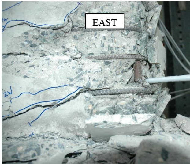
Figure 4-61 Photographs of observed fracture of longitudinal steel reinforcement at Cycle 39W Wall 2
