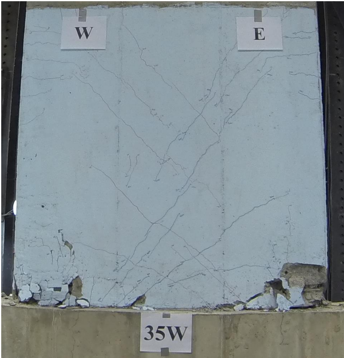
Figure 4-93 Wall condition at the peak of Cycle 35W on the South side Wall 3
