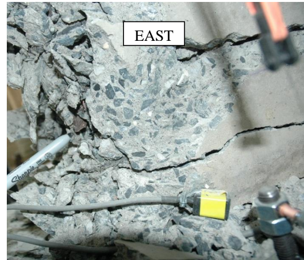
Figure 4-61 Photographs of observed fracture of longitudinal steel reinforcement at Cycle 39W Wall 2
