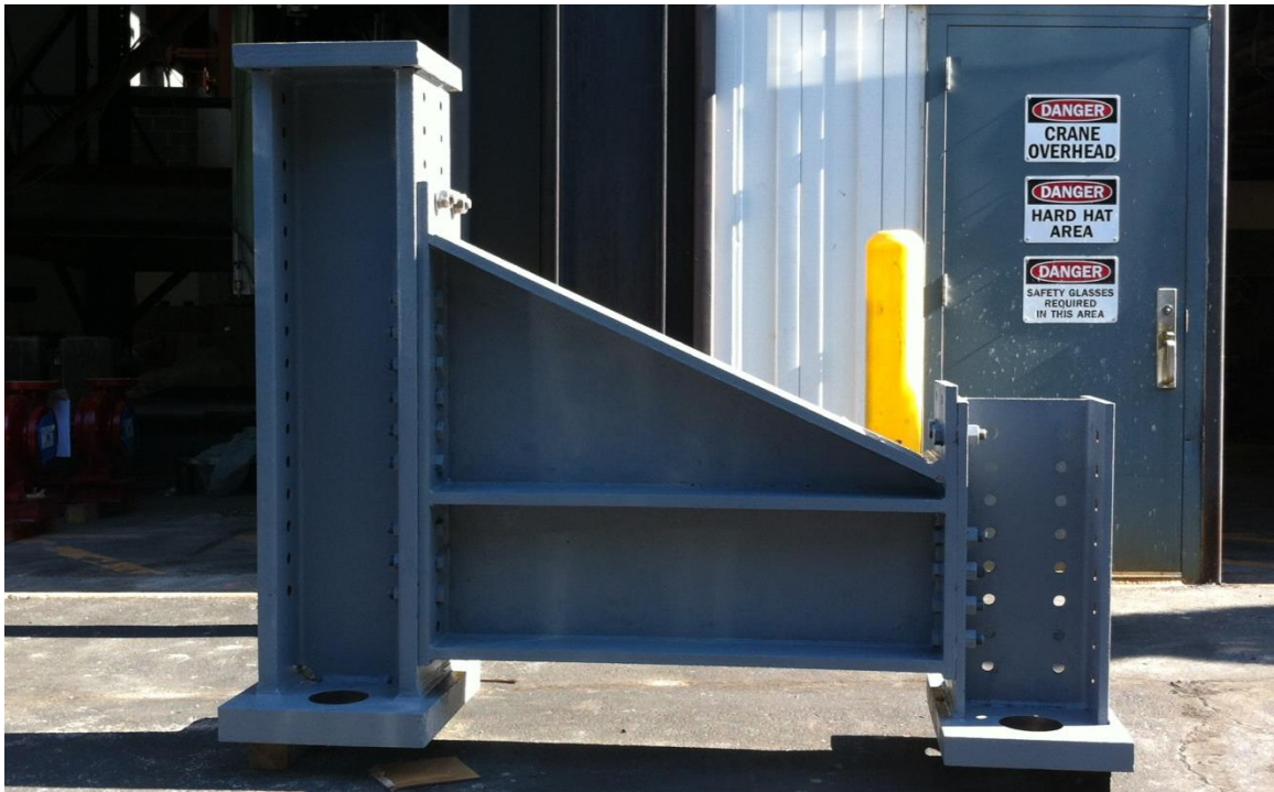
Figure 3-26 Actuator support fixture
