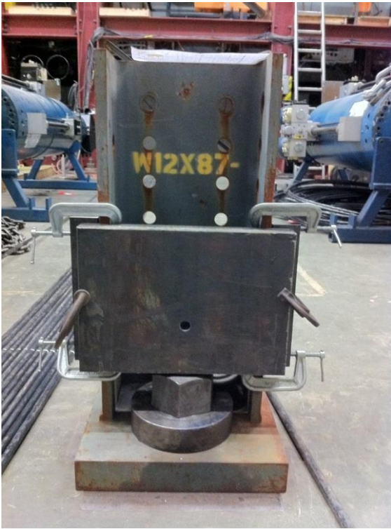
Figure 3-25 Setup for seating post-tensioning anchors
