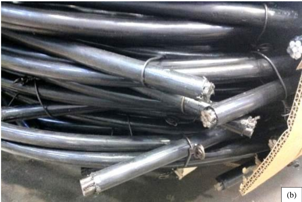
Figure 3-15 (a) PVC conduit that carries the unbonded post-tensioned tendons; and, (b) greased and sheathed strands
