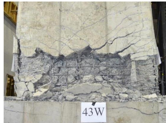
Figure 5-34 Photographs of progression of shear failure
