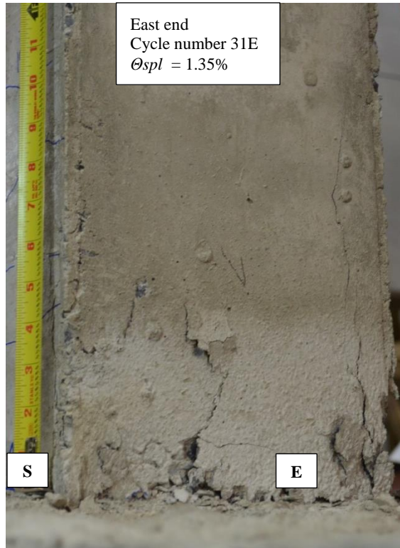
Figure 5-24 Initiation of observed spalling during Loading Step 11, Cycle 31
