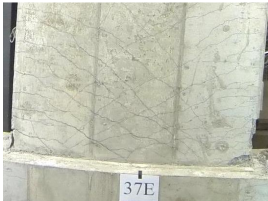
Figure 5-34 Photographs of progression of shear failure
