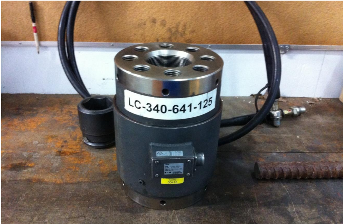
Figure 3-40 Load cell attached to the actuator
