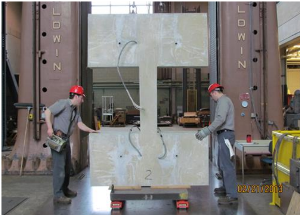
Figure 3-49: Transferring test specimens using rollers
