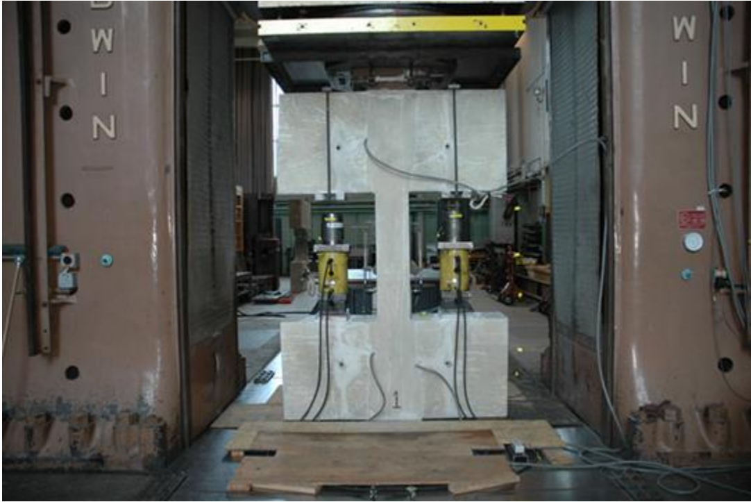
Figure 3-50: West face of TS01 before loading
