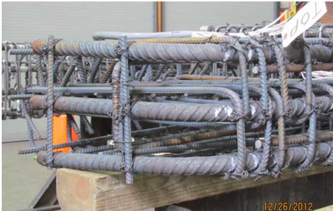
Figure 3-40: 90-degree hook of flexural bars
