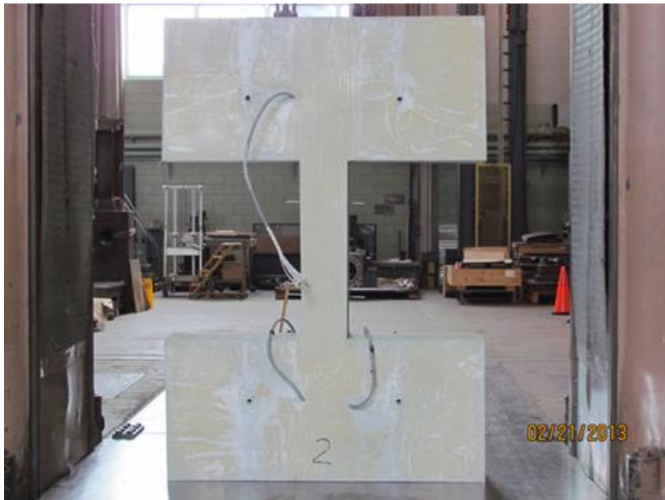
Figure 3-51: West face of TS02 before loading
