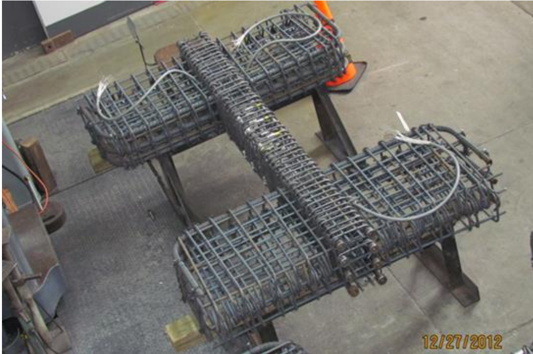
Figure 3-35: Reinforcement of TS01
