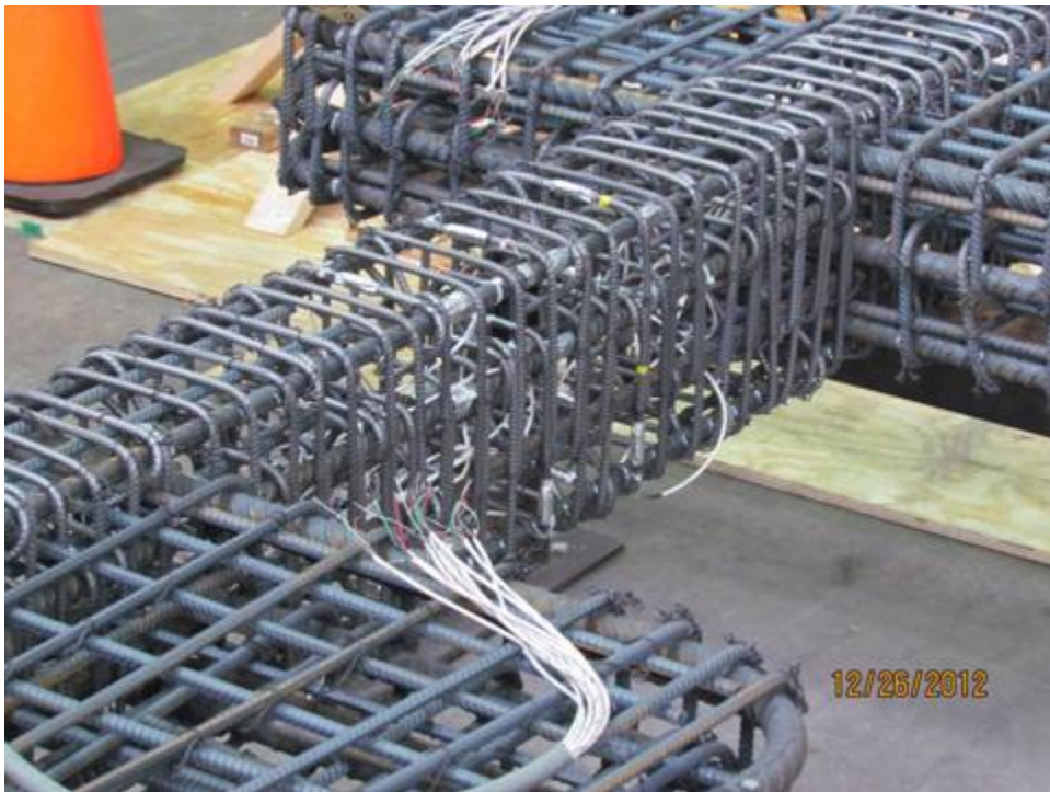
Figure 3-38: Strain gage instrumentation
