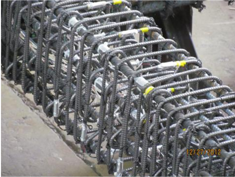
Figure 3-37: Strain gage instrumentation
