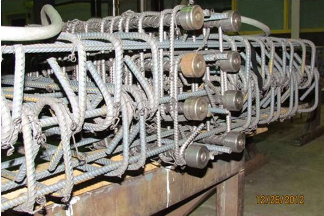
Figure 3-39: Headed bars used in confined concrete column
