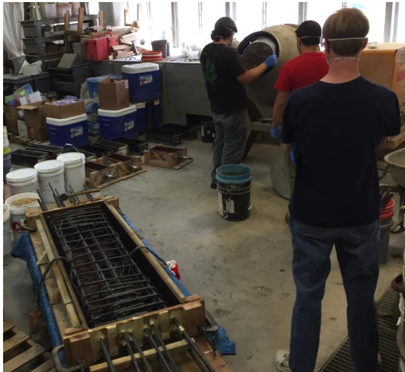
Figure 2.8: Mixing FRC and Coupling Beam Specimen Ready for Casting
