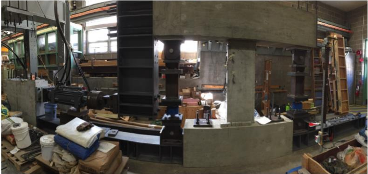
Figure 2.12: Coupling Beam Test Setup
