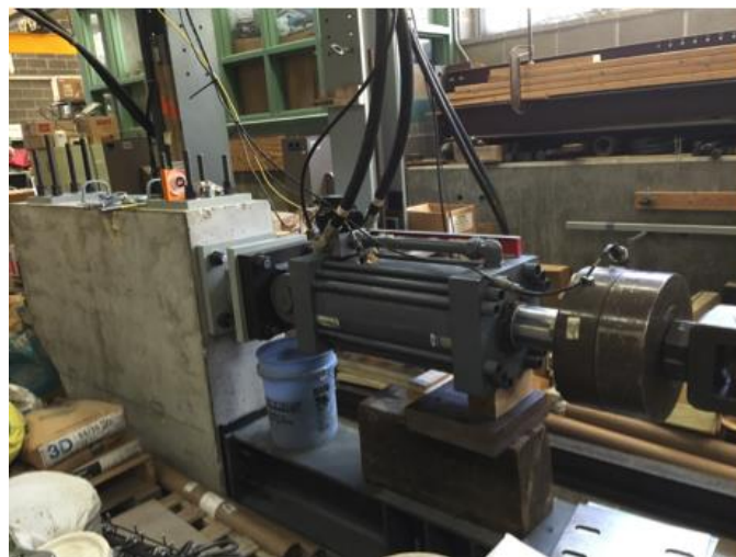
Figure 2.13: Hydraulic Actuator Connected to Concrete Reaction Block
