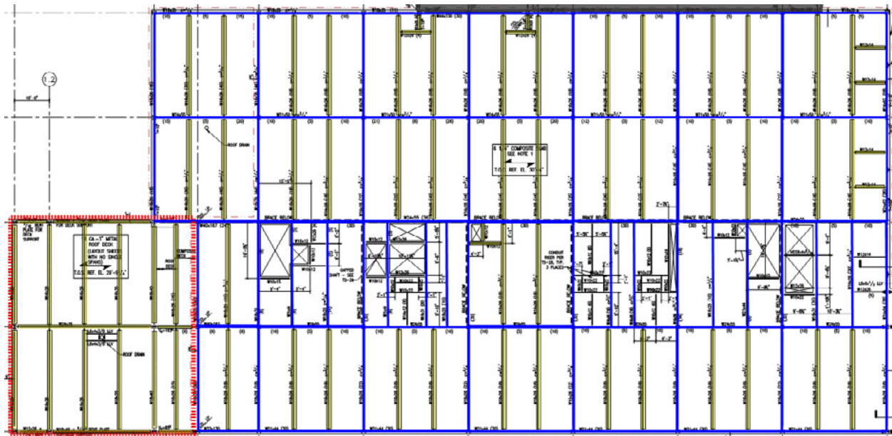
Figure 7-46. Design 3 Structural insulation distribution (Level 3 framing).
