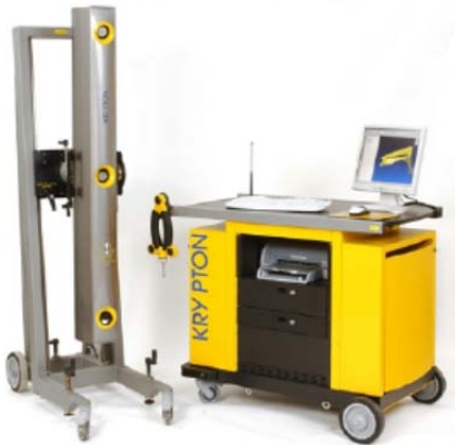
Figure 5.10: Nikon Metrology/Krypton K600 Optical CMM System
