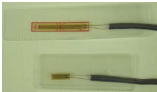
Figure 5.2: Concrete surface gauge (above) and steel reinforcement gauge (below)
