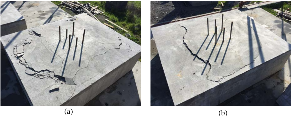
Figure 5 – Overhead view of breakout surface for (a) 12-inch embedment and (b) 18-inch embedment
