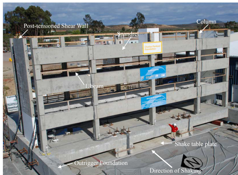
Fig. B4-1. Shake table testing specimen (Modified from Schoettler et al. 2009).
