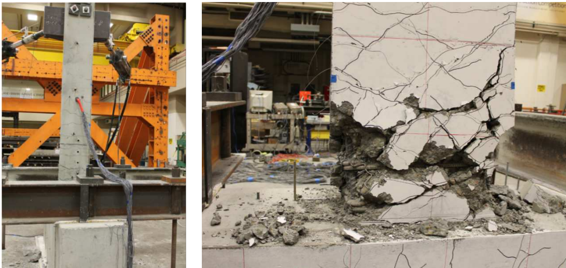
Figure 3.3.1: Failure Mechanism of SBH60 by Twisting of Beam (Global Instability)
