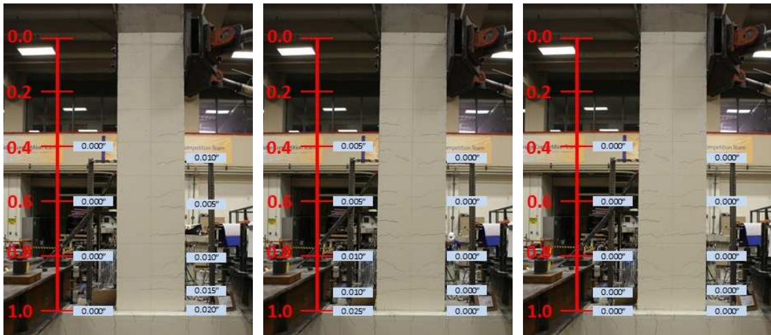
Figure C-16: Measured Crack Widths at Drift Ratio of 0.6% – Specimen SBL100
