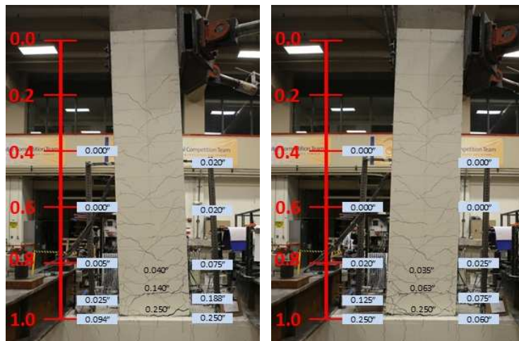
Figure C-22: Measured Crack Widths at Drift Ratio of 4.85% – Specimen SBL100
