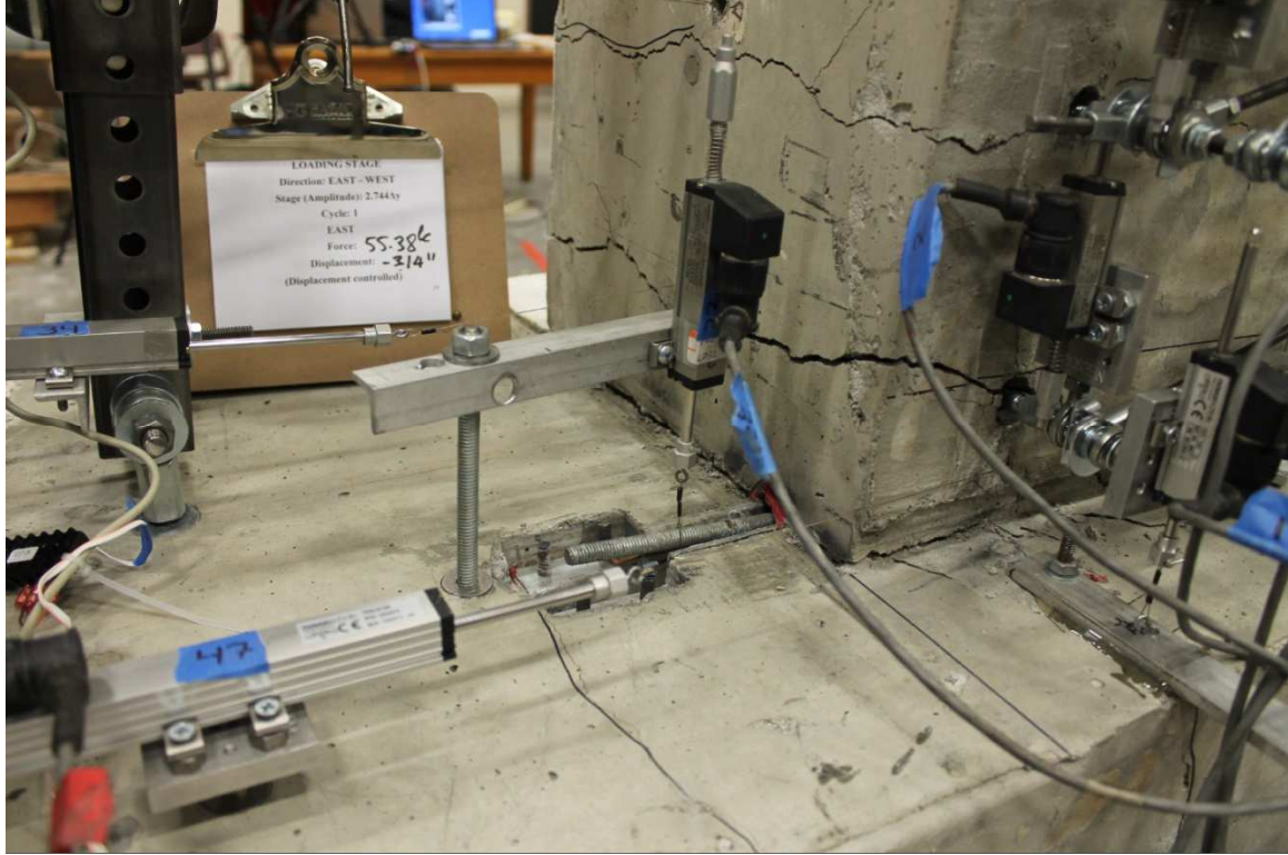
Figure A-21: General Instrumentation for Measuring Slip by Brass-Brazed Threaded Rods
