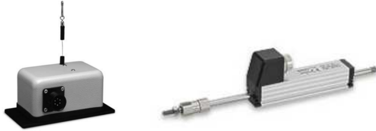
Figure A-11: Typical Displacement Transducers Used in Tests. Left: String Potentiometer for Global Deflection Measurement; Right: Novotechnik Used to Measure Local Deformations
