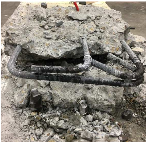
Figure 3.3.4: Failure Mechanism of SBM100 by Fracture of Longitudinal Bars
