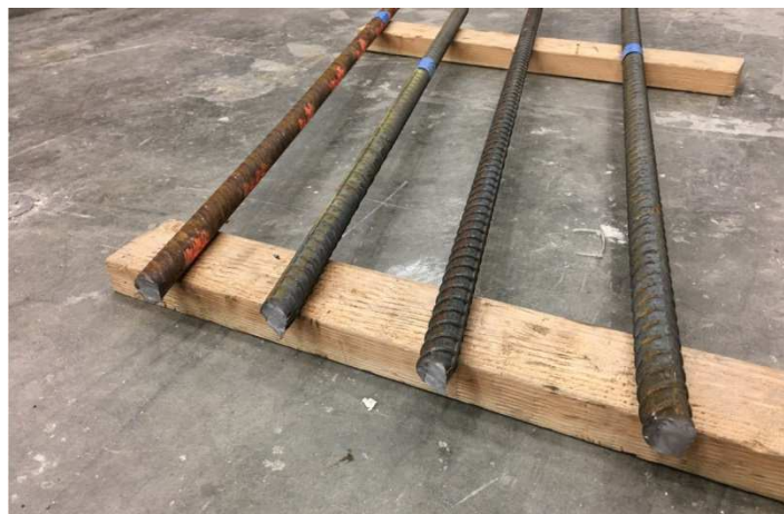
Figure A-5: Longitudinal Steel Used in Test Specimens - Left to Right: SBL100, SBH100, SBM100, SBH60
