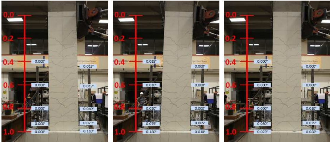
Figure C-20: Measured Crack Widths at Drift Ratio of 2.45% – Specimen SBL100
