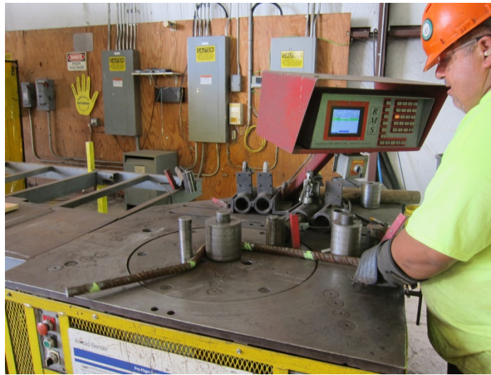
Figure 3: RMS Arnold Bender used to bend specimens
