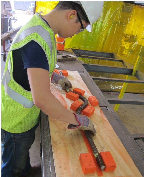
Figure 4: Verifying bend specimen tolerance
