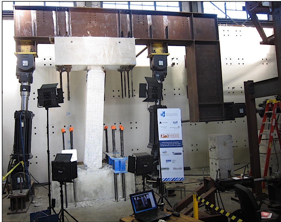
Figure 12: Column CL100 at the end of the test
