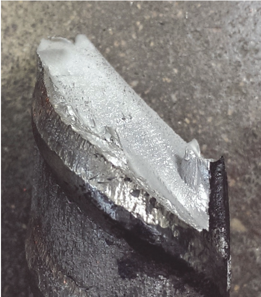
Figure 34: Photograph of a fractured bar where the fatigue crack initiated at, and propagated along the base of a transverse deformation.
