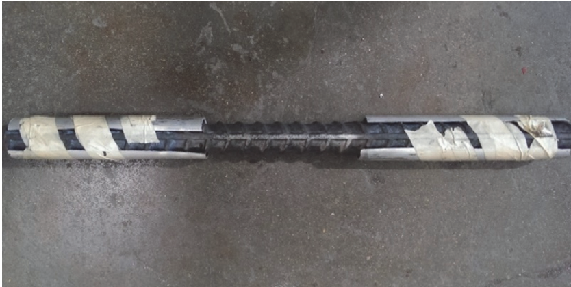
Figure 4: Aluminum tubing temporarily attached to the ends of a bar with tape.
