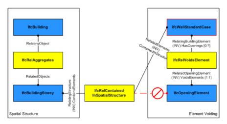
Figure 15 Relation between a wall and an opening in IFC through the objectified relationship IfcRelVoidsElement.
