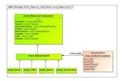
Figure 23 Detail of inheritance structure for mwd\_MasonryUnit. Preliminary list of most common masonry unit component types.
