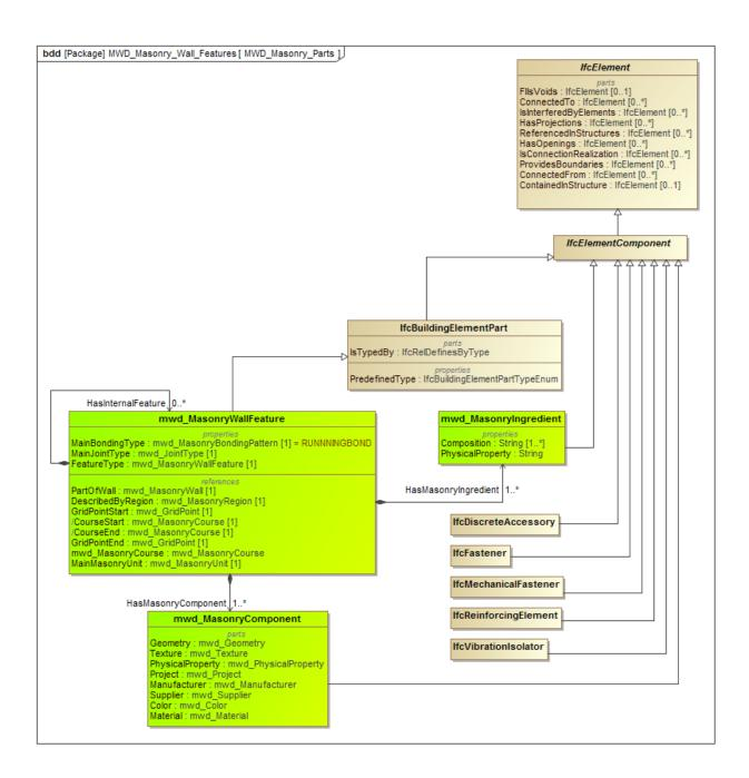
Figure 20 Proposed inheritance structure for masonry features, components and ingredients.
