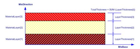
Figure 16 Structure of Material Layer Set.
