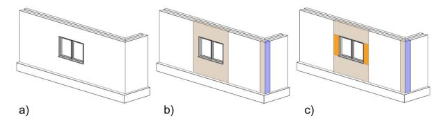
Figure 1 Region top-down decomposition according to the insertion of a window opening.
