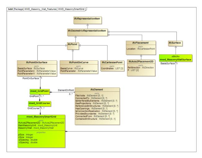
Figure 28 Definition for a smart masonry wall grid.
