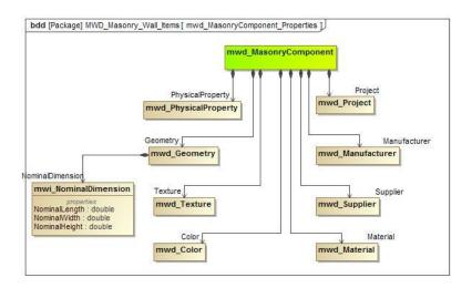
Figure 21 Shared properties for all mwd\_MasonryComponent, based on MUD.
