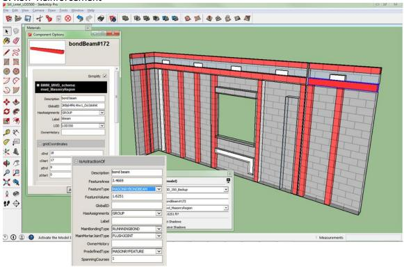
Figure 43 Region representation of a bond beam section.
