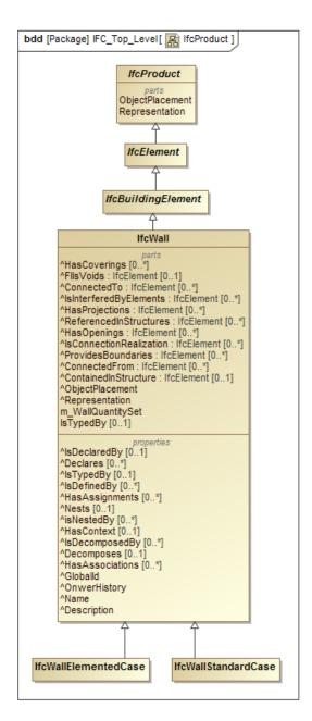
Figure 17 Inheritance structure for IfcWall, IfcWallStandardCase and IfcWallElementedCase.
