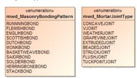
Figure 26 Enumerations for main bonding pattern type and mortar joint type.
