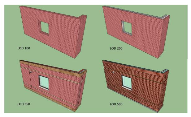
Figure 32 Sequence of LODs for masonry wall model.
