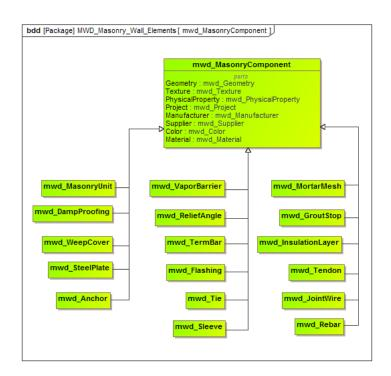
Figure 22 Preliminary list of most common masonry component types.
