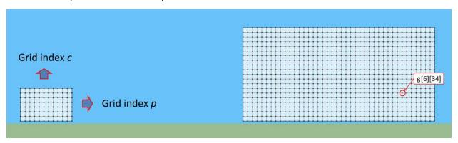
Figure 35 Definition of a Masonry Smart Grid object. The underlying geometric representation could be a surface with a UV mesh for indexing the position of smart point objects.
