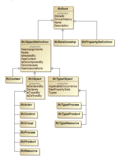
Figure 12 Basic IFC definitions, using SysML block diagrams.
