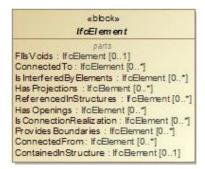
Figure 14 Inverse attributes defined for IfcElement and its subclasses.
