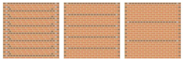
Figure 5 Brickwork patterning. Each sub-pattern may be depicted as brickwork region with specific information associated (e.g. color, texture, and manufacturer). Images by Jonathan Riley, available under Creative Commons license.
