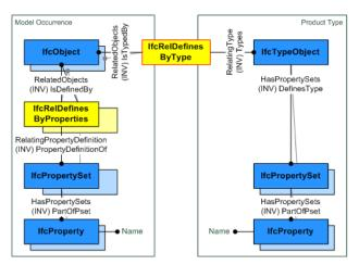
Figure 13 Assignment of a predefined product type to an object occurrence using IfcRelDefinedByType objectified relationship.
