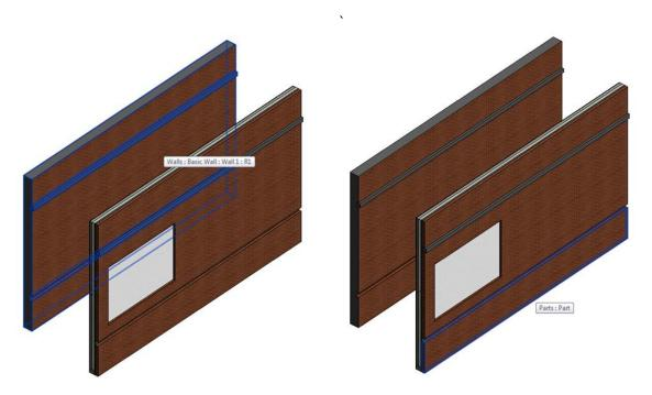
Figure 18 Models of masonry cavity wall in Revit 2015. In the left wall, all layers and masonry features are implicit in the model (e.g. material layer set) created as a Revit stacked wall. This representation is similar to IfcWallStandardCase. On the right, all layers and features are represented explicitly as independent parts of the wall, which is equivalent to IfcWallElementedCase.
