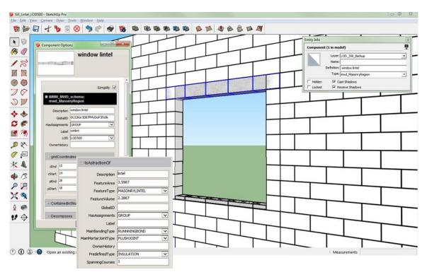
Figure 39 Lintel and sill, depicted by regions at LOD 500. A second set of fields allows the specification of the region as abstraction of a masonry sill (FeatureType property). The uppercase MASONRYFILL is part of an enumeration of predefined masonry feature types.
