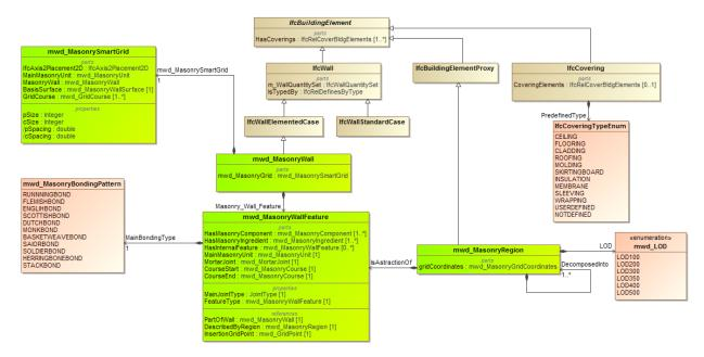
Figure 30 Relationships between mwd\_MasonryWall, mwd\_MasonryWallGrid, mwd\_MasonryWallFeature and mwd\_MasonryWallRegion. A mwd\_masonryWallRegion is an abstract, proxy representation of a masonry feature that has a LOD associated to it.
