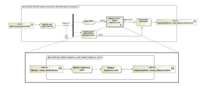
Figure 34 Overall workflow in setting a Masonry Smart Grid. Bottom half of the figure shows the internal activity of selecting a masonry unit from MUD.
