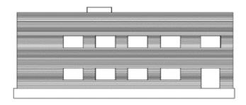
Figure 10 Schematic regions for quantity take-off based on masonry courses.
