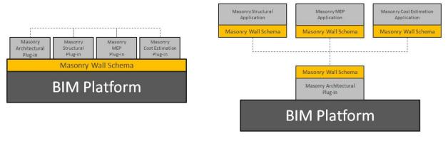
Figure 31 Plug-in architecture for internal or external application integration. On the left a plug-in architecture.
