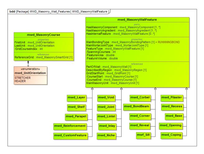
Figure 27 Preliminary list of masonry wall features. Each feature indirectly refers to the masonry wall grid (mwd\_MasonrySmartGrid) through its insertion points specified by the properties GridPointStart and GridPointEnd. The courses where the feature starts and ends are derived properties calculated from the insertion points.. Each masonry course knows if its first masonry unit is a header or a stretcher, based on the main bonding pattern of the wall.
