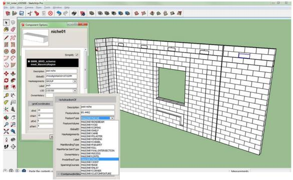
Figure 41Region representation for niche to receive roof joists.
