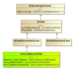
Figure 19 Masonry walls as subtype of elemented walls/
