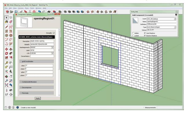
Figure 36 Characterization of a window opening in a CMU backup wall according to the Masonry Wall Definition schema.
