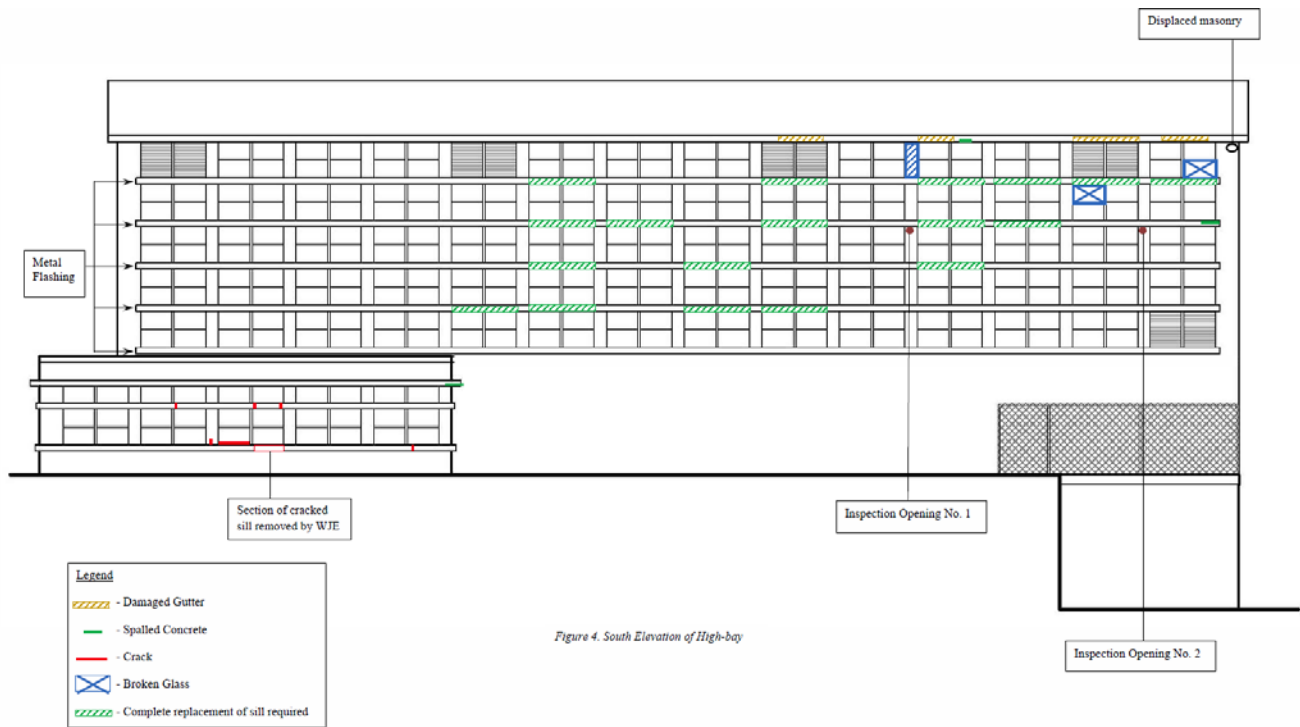
Figure 9-22. Noted elevations for repair.
