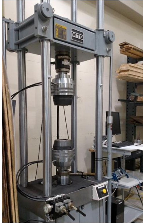
(a) MTS universal testing machine
