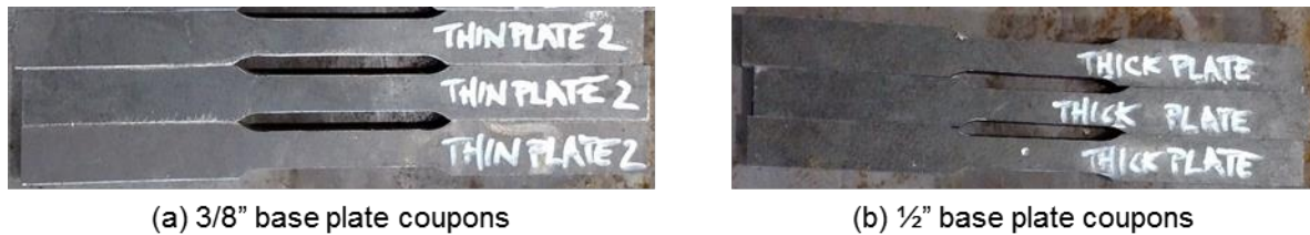
Figure A-56: Photographs of base plate coupon specimens
