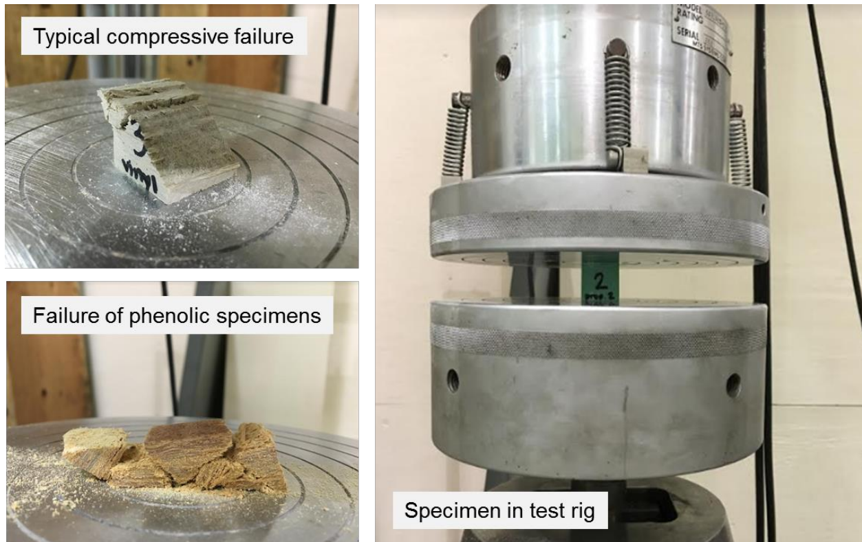
Figure A-76: Photographs of typical failure modes and test setup in MTS universal testing rig
