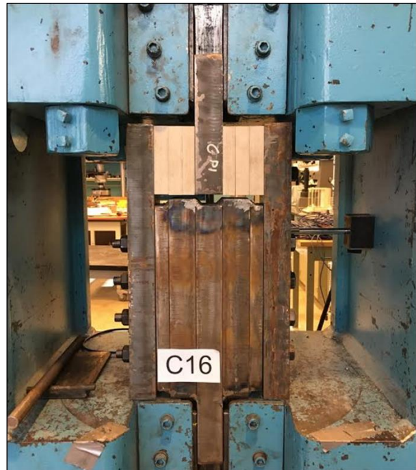
Figure 5-1: Schematic of test rig and photograph of specimen C16 (3" vinylester shims) installed in universal testing machine
