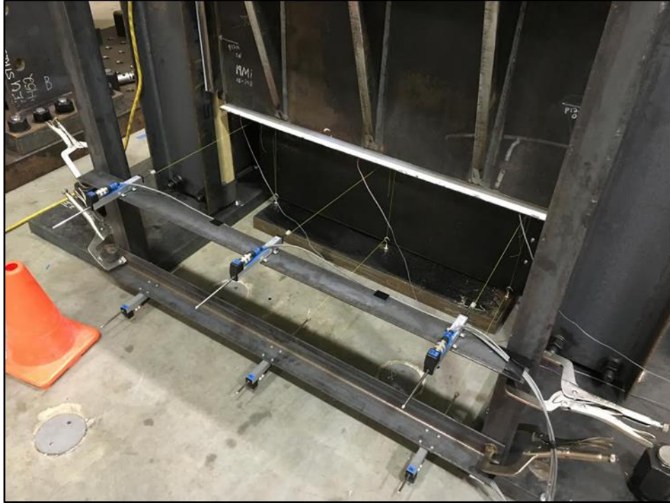
Figure 6-5: Photograph of experimental setup, depicting horizontal position transducers D1-D3 in top row, and vertical position transducers D4-D6 in bottom row, both mounted to rigid frame.
