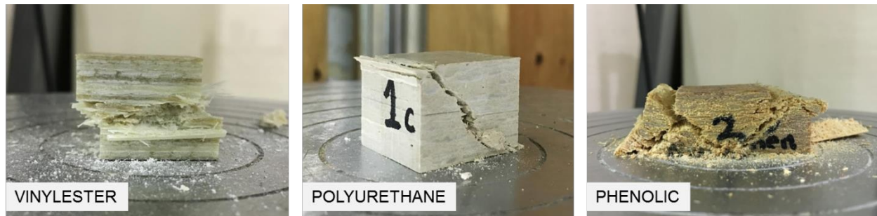
Figure 4-1: Typical failure modes for (a) vinylester (b) polyurethane, and (c) phenolic resins.
