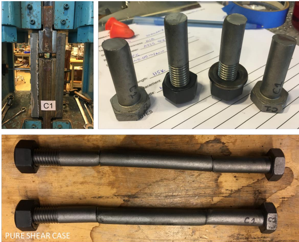
Figure 5-8: Photographs of post-failure specimen bolts from test C1
