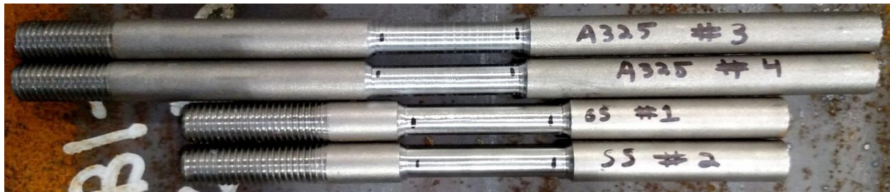
Figure A-60: Photograph of A325 (#3 and #4) and A304-SH1 (#1 and #2) specimens prior to testing
